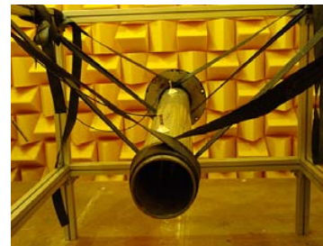
Fig. 6. Photograph of the test duct installed in the full anechoic chamber for the investigation of the acoustic propagation characteristics.
